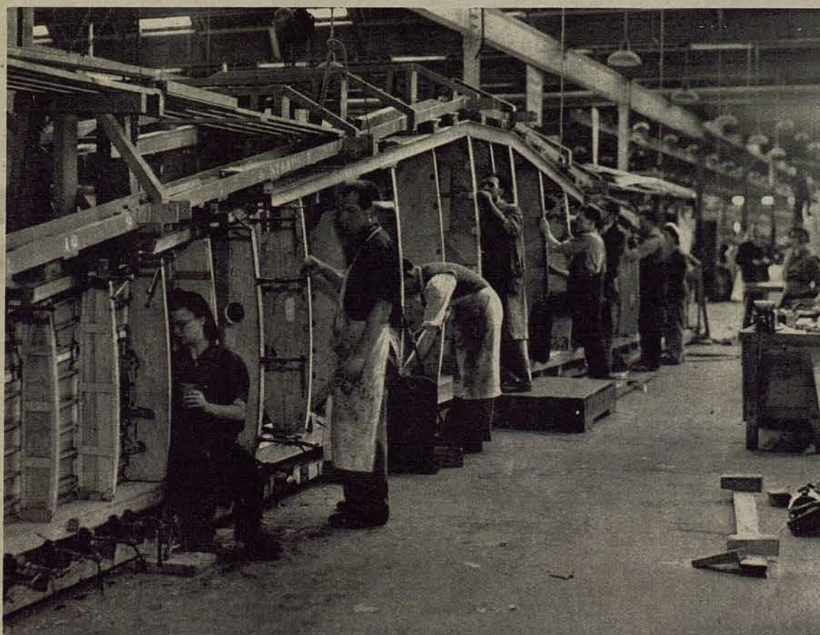
9 A Different Log Lends a Hand to Form the Spars and Ribs The spars are made of spruce imported from the Pacific seaboard of Canada and America. Spruce was the timber used when flying was in its infancy.
