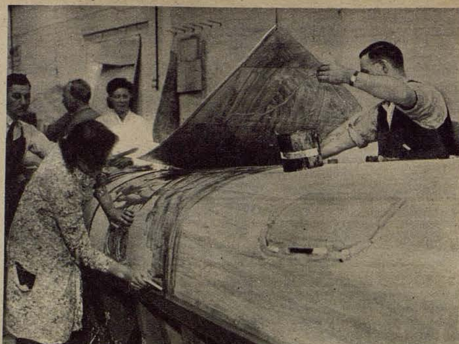
12 The Fuselage Shell is Built in Two Halves Over the plywood, now wrapped round the jig, thick strips of balsa wood are cemented. Then comes the second plywood skin.
