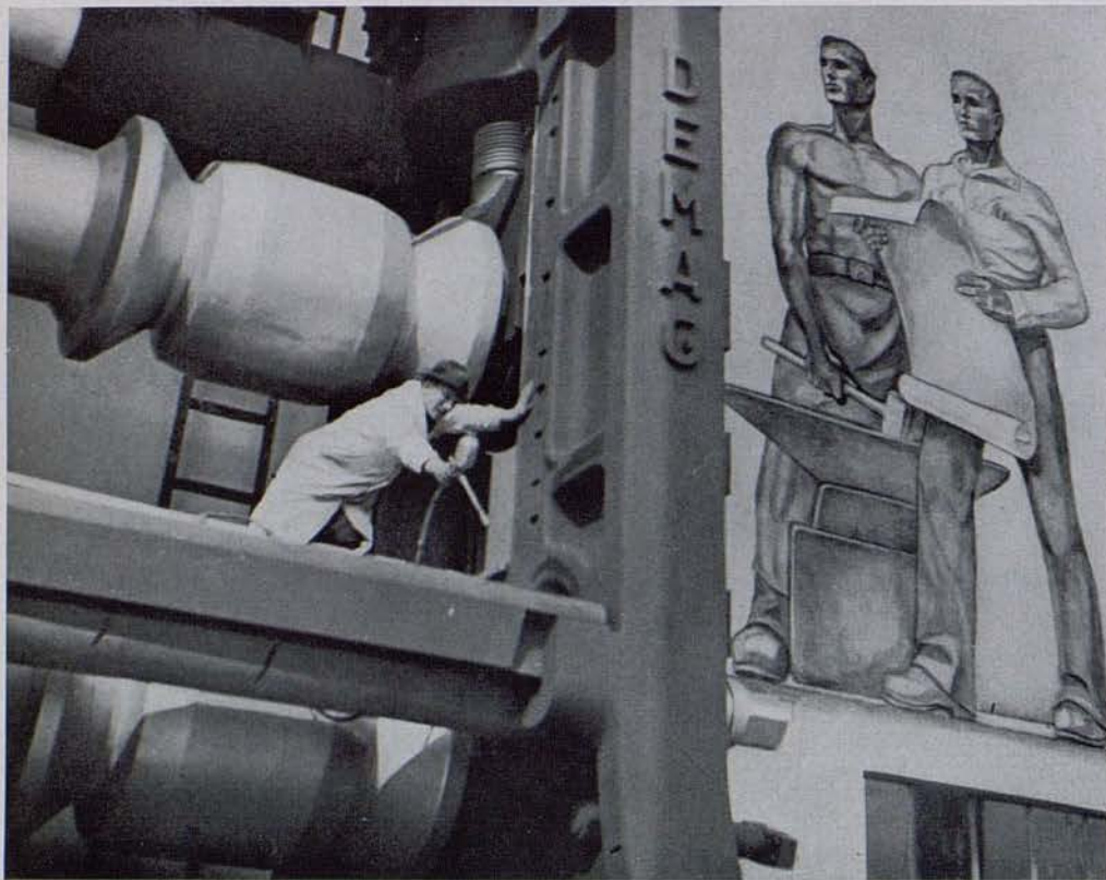
The DEMAG displayed an exact replica of a reverse rolling mill, 37 feet high
