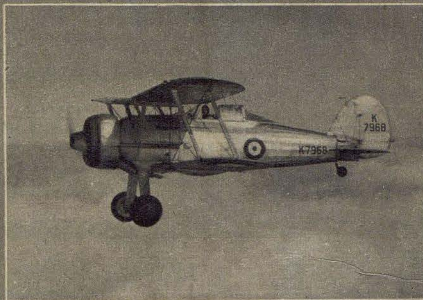
Gladiator 255-m.p.h. four-machine-gunned Fighter and Sea-Fighter.
