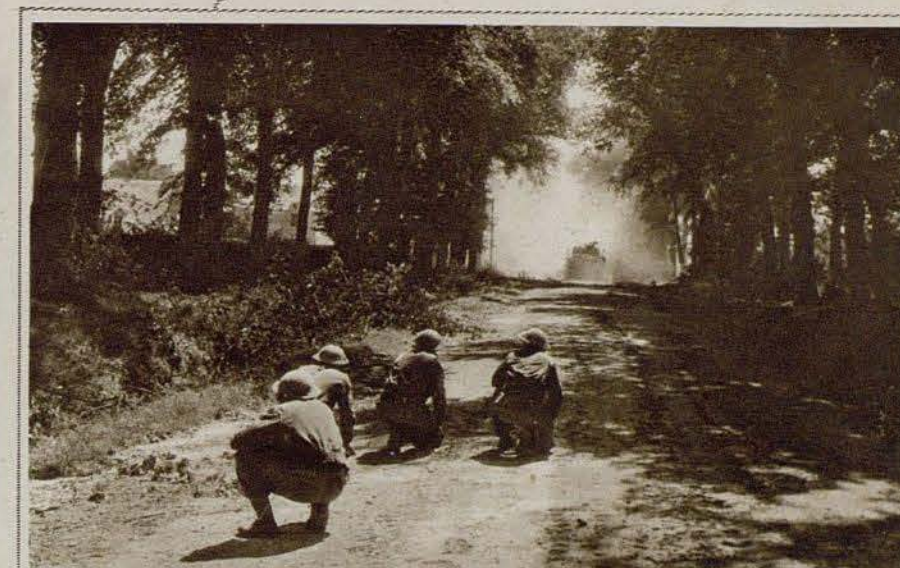
A FLAIL TANK AT WORK CLEARING MINES OFF A ROAD: IN THE FOREGROUND ARE ENGINEERS WAITING TO GO FORWARD.
