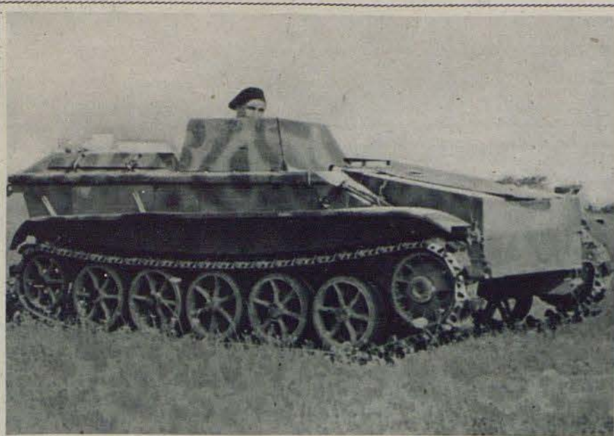
THE GERMAN V-4 ROBOT TANK. IT HAS A DRIVER FOR A CERTAIN DISTANCE BEFORE BEING DIRECTED BY WIRELESS. THIS TANK WAS CAPTURED ALMOST INTACT DURING OUR ADVANCE IN NORMANDY.
