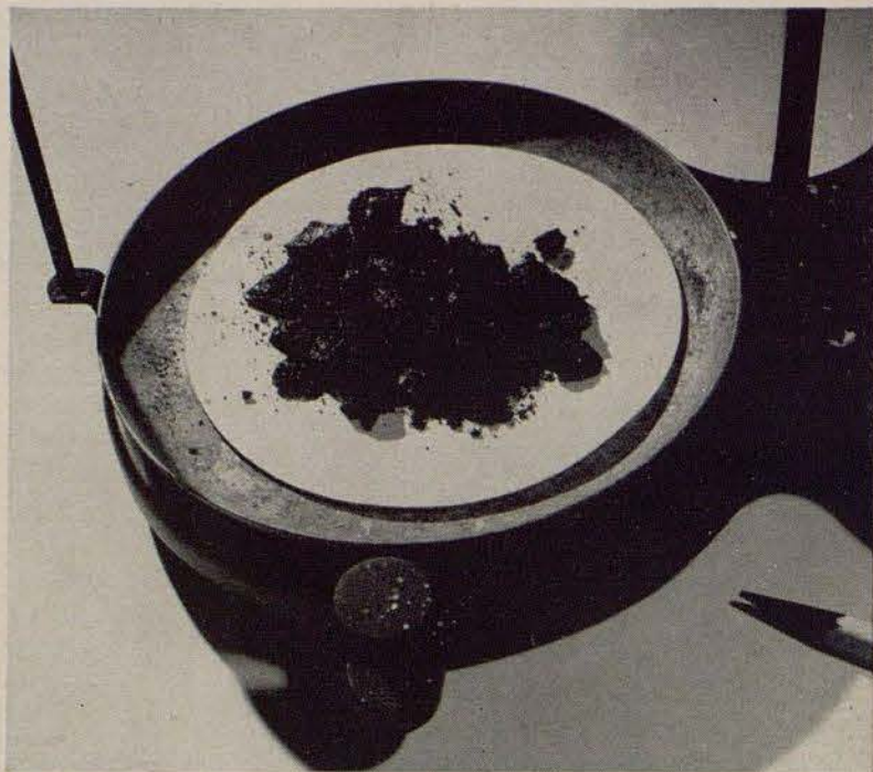
Synthetic coal, produced in laboratory, in appearance and in exact chemical analysis is identical with natural bituminous coal. From it Dr. Berl has made hard coke.
