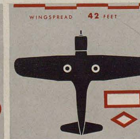
SB2U looks like the F4U (above). Its squarish wing and wingtips set it off, although the diamond tail is the same.
