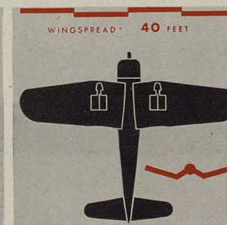
F4U can be told by its inverted gull wing which stands out at almost any angle. The other clue is the narrow tail.
