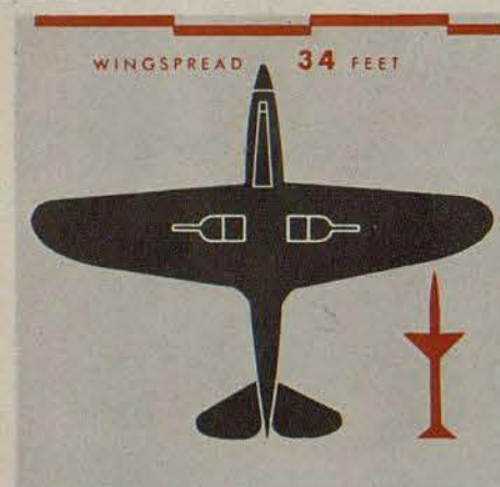
P-39 is easy to spot by its long, narrow, pointed nose. Other clues—the high cabin, air-scoop hump—show up in side view.
