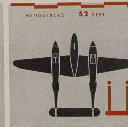
P-38 can't be mistaken for anything else. Its long narrow tail and its two rudders trail out behind, supported on two booms.
