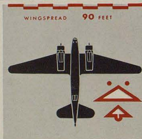
B-23 looks like the B-18A. Differences are longer tail with gunner's post at the end, shallow fuselage and rounded nose.
