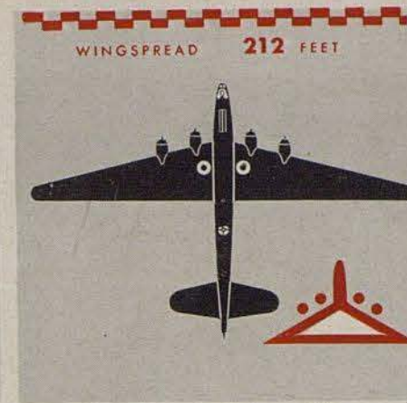
B-19 has an ordinary tail. It is spotted by its long front-pointed triangular wing, its long nose, its tremendous size.
