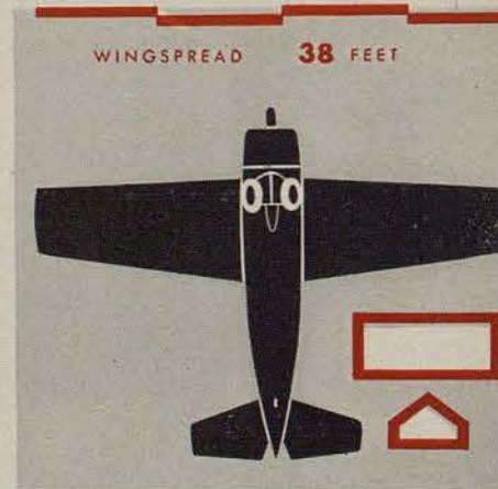
F4F is recognised by its square wing and its squared-off tail. Like most U.S. war planes, its motor is air-cooled.
