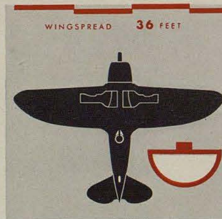
P-43 with its air-cooled motor, stubby nose, has a wing that curves back from the leading edge like a meat chopper.
