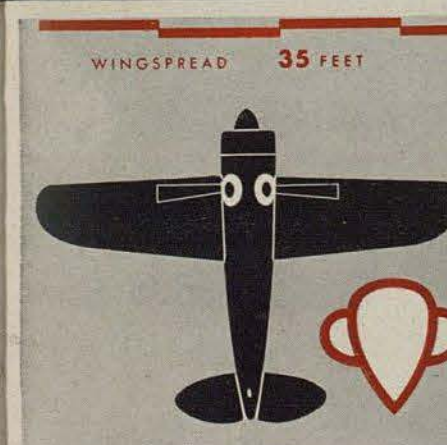
F2A with its roly-poly fuselage, looks like the F4F, but the smooth curves of the wingtips and tail set it off.
