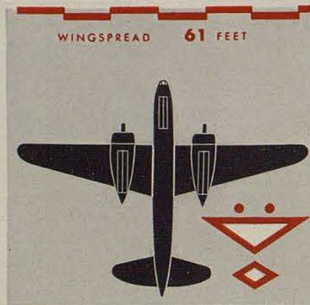
A-20A has its triangle wing pointing backwards. Single-rudder tail is diamond-shaped. The plane has humpback.
