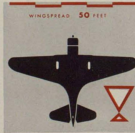
TBD is distinctively marked by its very deep triangle wing, tapering back all the way to the opposite triangular tail.
