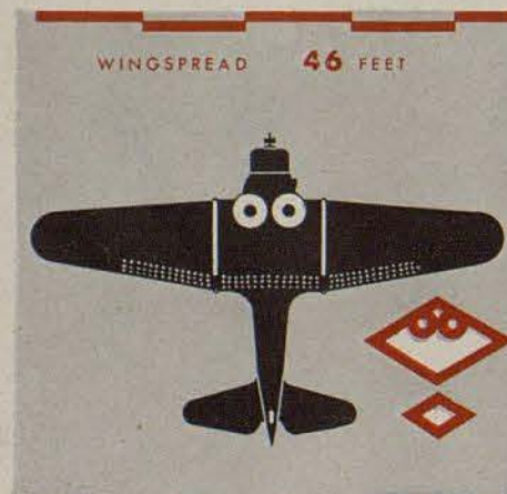
A-17A looks like the SBD and the A-24, with its double-diamond form. Its wheels tucked together and small nose are clues.
