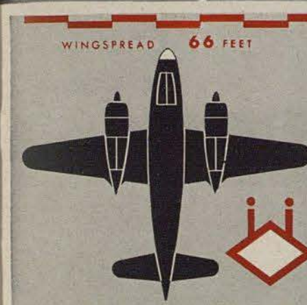
B-26 with a diamond-shaped wing, has its big motors far out in front of the leading edge in long nacelles.
