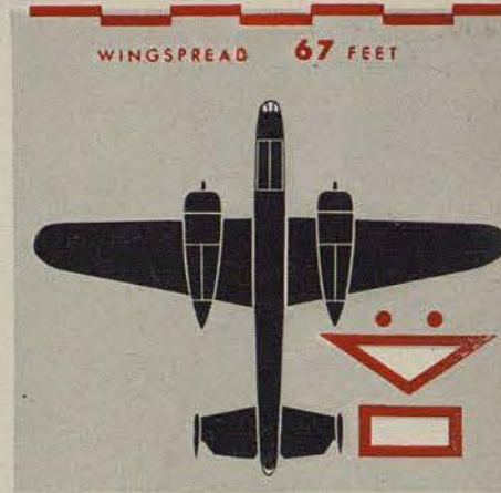
B-25 has wing like A-20A. Difference between planes is in tail, where the double rudders give square outline.
