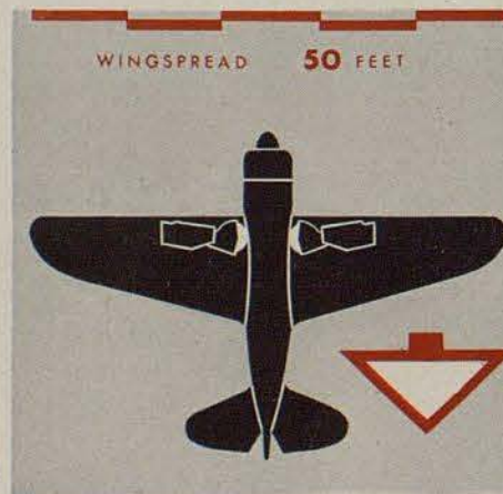
SB2C has the typical Curtiss triangular wing (see above) but can be told from the P-40 by its squared nose.
