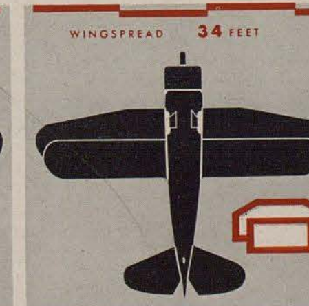
SBC is another of the rare biplanes. Upper wing's sharp sweepback is the clue here. Plane's fuselage is also longer.
