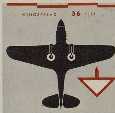
P-40 also has a pointed nose, but not so long and narrow as the P-39. The nose and triangular Curtiss wing are its marks.
