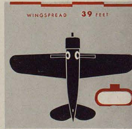
SBN has the same rounded Brewster wing as SB2A and F2A. Short nose and slim fuselage settle its identity.
