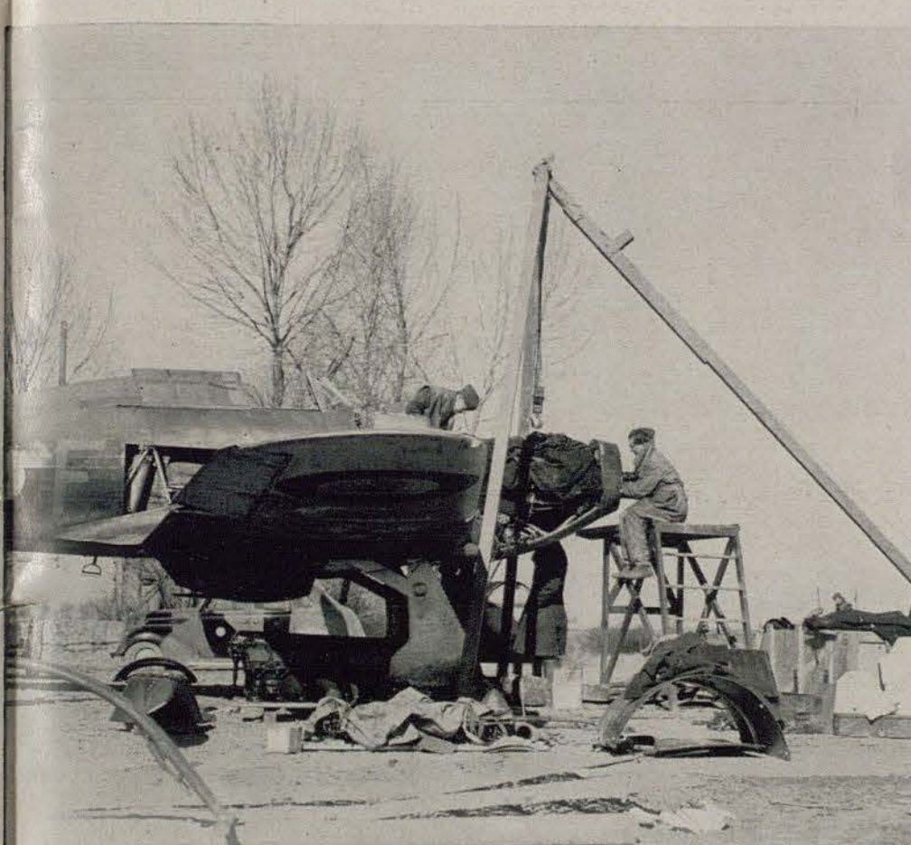
Somewhere in France the maintenance men of the R. A. F. are pulling an engine from a Hurricane for overhauling. Most Hurricane fighters are based in France. Spitfire fighters are based in Britain.
