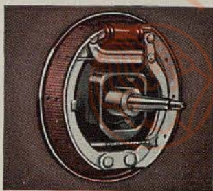
BIG HYDRAULIC BRAKES: Largest drums and lining area of any low-price car—for fast, straight-line stops and long service. Pedal action smooth and easy.
