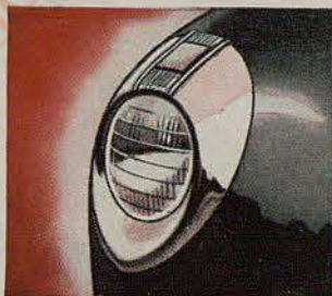
SEALED-BEAM HEADLAMPS: Light is much stronger, stays bright longer. Night driving safer and easier. Bulb, lens and reflector all sealed in single unit.
