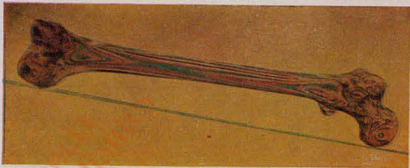
TRANSLUCENT THIGHBONES carved out of photoelastic plastic produce distinct light patterns during strength tests. Stress lines frozen into these models
