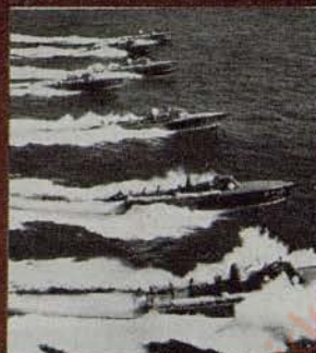
UNCLE SAM'S HARD-HITTING PT BOATS are made of light, wood construction for high speed, strength and maneuverability.
