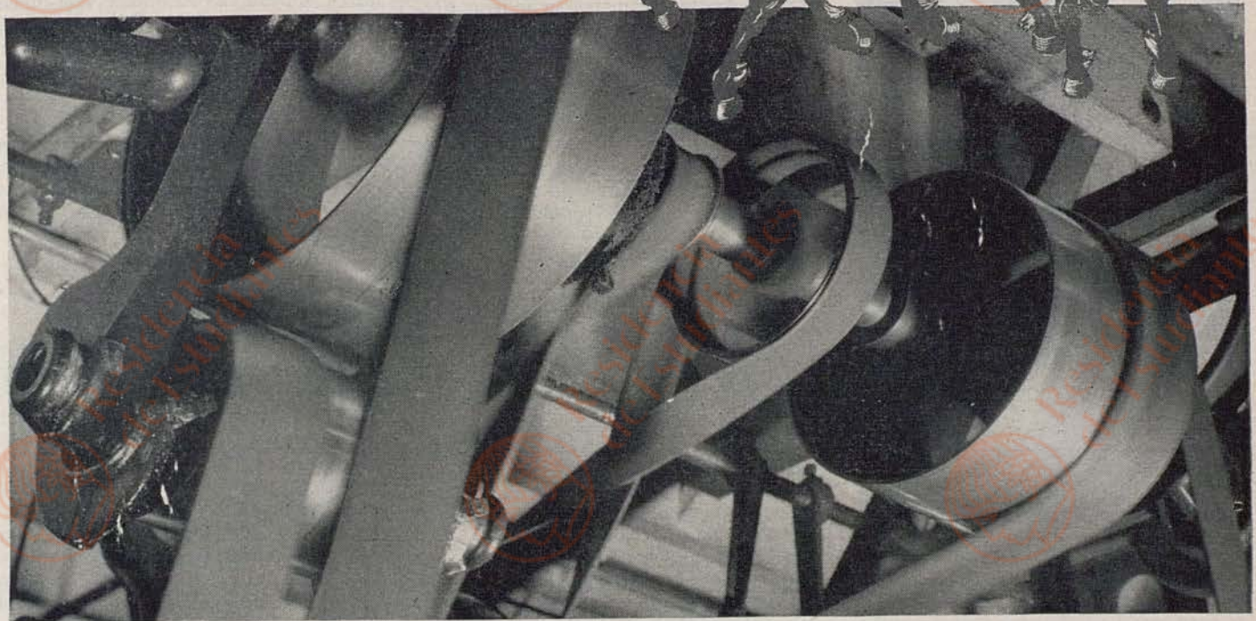
HEWITT Factory-Built Endless Transmission Belts have a special drum splice which eliminates any break, lapped or cemented joint.
