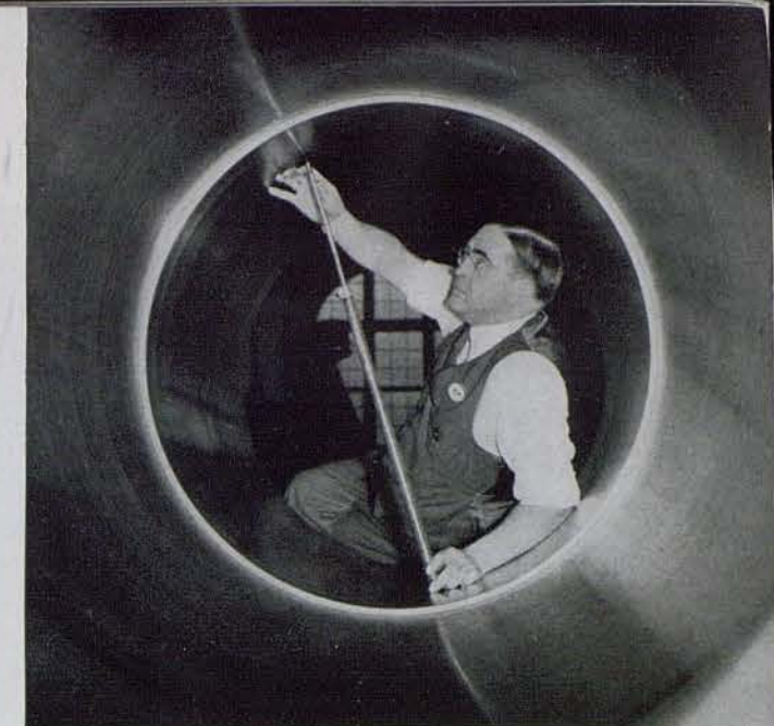
Measuring with micrometer inside a big gun barrel.
