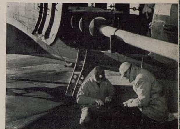
Aerial wire-laying was achieved this year by ATSC and Signal Corps men who devised device, shown here on C-47, that can lay wire across any kind of terrain within 16-mile range in 60 minutes.
