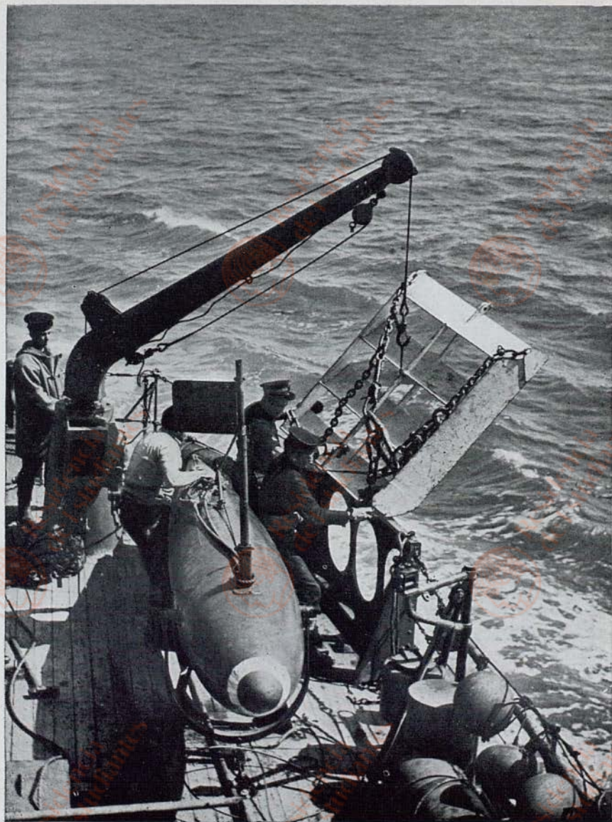
The sweeping apparatus is lowered from mine-sweeper to sea by means of a crane.
