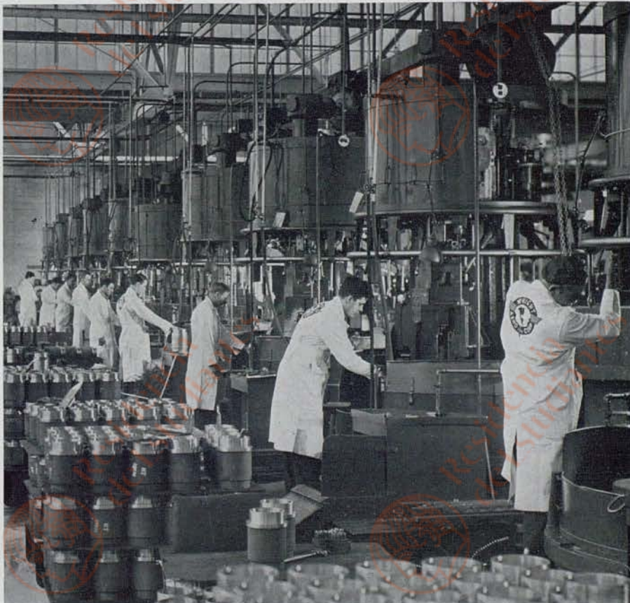
BATTERY OF "MULT-AU-MATIC" machines for turning, facing and boring Cyclone cylinder barrels. Weighing 15 tons these 14' machines each replace several single-purpose machines.
