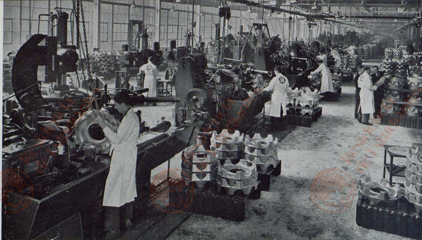
OPERATORS USING fastematic turret lathes to machine the inside and outside surfaces of crankcase sections.
