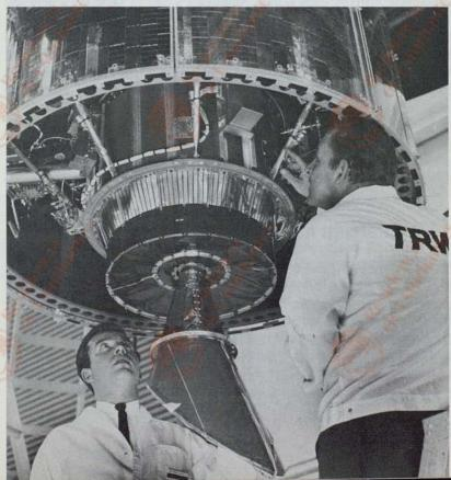
doughnut-shaped omnidirectional telemetry and command antenna. Two axial thrusters mounted aft, two radial thrusters mounted at side. Earth and sun sensors mounted at side. Supporting subsystem equipment mounted inside on circular aluminum honeycomb platform. Spin stabilized at 90 rpm. Weight at liftoff: 642 pounds.
