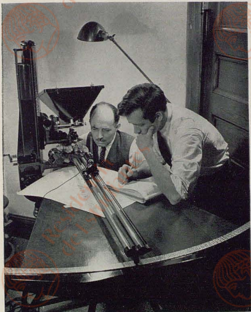
This plotting instrument, invented by Mr. O. M. Miller (left) of the Geographical Society, makes it comparatively easy to plot maps of mountainous country from aerial photographs. The pencil that draws maps is supported on the two long bars.
