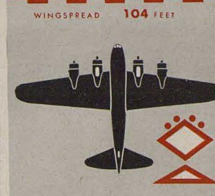
B-17 has a fat diamond wing, and a triangular tail. The fuselage is round and thick, and the short nose is gently rounded.
