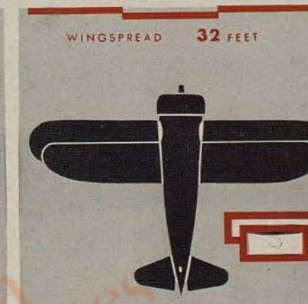
F3F is easy to spot. One of the few biplanes still flying with the Navy, its fuselage is short, chunky and deep-bellied.
