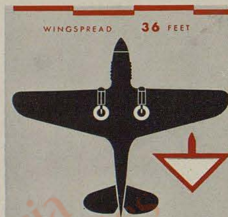
P-40 also has a pointed nose, but not so long and narrow as the P-39. The nose and triangular Curtiss wing are its marks.
