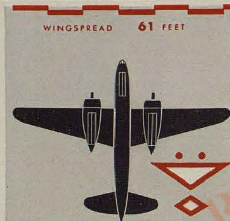
A-20A has its triangle wing pointing backwards. Single-rudder tail is in tail, where the diamond-shaped. The plane has humpback.
