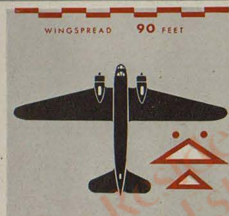
B-18A is recognised first by its front-pointed triangle wing. Other clues: a deep-bellied fuselage and a shark-like nose.
