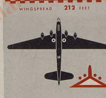
B-19 has an ordinary tail. It is spotted by its long front-pointed triangular wing, its long nose, its tremendous size.
