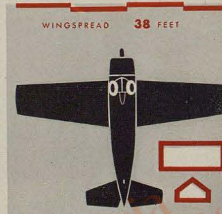
F4F is recognised by its square wing, its squared-off tail. Like most U.S. war planes, its motor is air-cooled.
