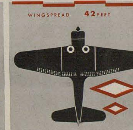
SBD is a dive bomber. Identifying marks are its diamond wing and tail. Swiss-cheese flaps open in dive and are easily seen.
