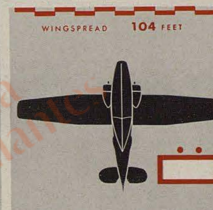
PBY-5 is the only square-winged two-engine plane. Like the PBM, it is a flying boat—blunt-nosed, thick-bodied.
