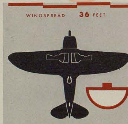
P-43 with its air-cooled motor, stubby nose, has a wing that curves back from the leading edge like a meat chopper.
