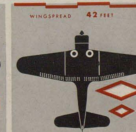
A-24 is identical with the SBD (above), but used by the Army. Double-diamond pattern means either the SBD or A-24.
