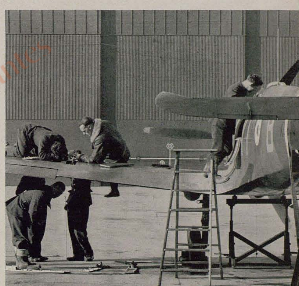
Lining up the guns of a Spitfire fighter is a precise and important job. These fast interceptors carry four machine guns in each wing. All together they can fire 160 rounds a second.
