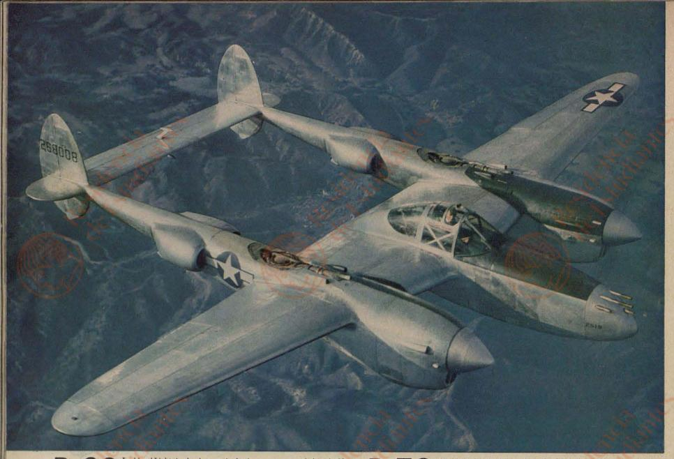
P-38 Lockheed Lightning has been revised to increase range and altitude. New aileron boosters improve the plane's climb and maneuverability. Besides its cannon and four machine guns, it now can carry two 1,000-lb. bombs.
