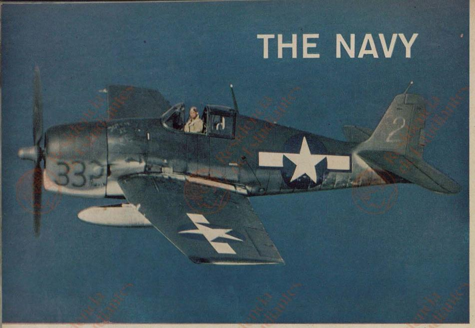
F6F Grumman Hellcat, the Navy's most widely used carrier fighter, is a low-winged development of their F4F or Wildcat. The bigger, supercharged engine takes it faster and higher, auxiliary gas tank extends its range.
