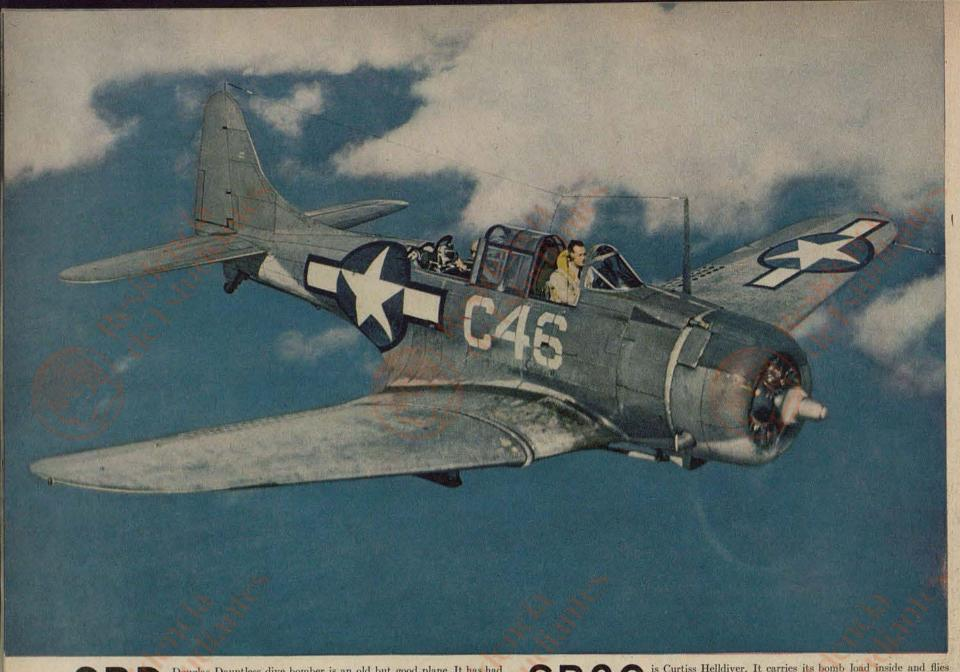
SBD Douglas Dauntless dive bomber is an old but good plane. It has had many improvements since first designed, most coming from combat study, including higher-powered engine, more guns, self-sealing tanks.
