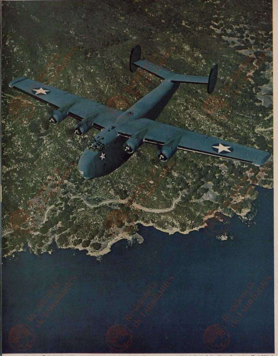
PB2Y is Navy's biggest patrol plane except for the behemoth Mars. These Consolidated-built Coronados have been used mainly as long-haul freight planes between Pacific bases. Modifications have been made to enable them to carry a
